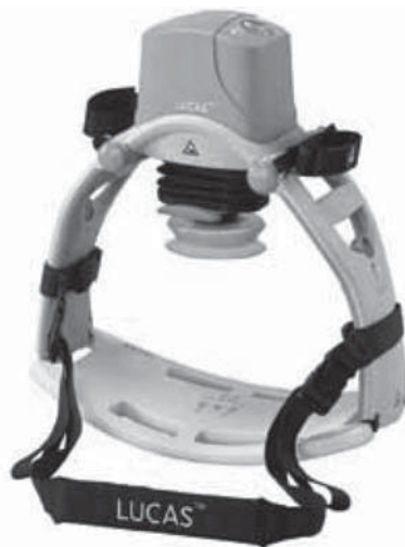
Figure 2. LUCAS Device. (Courtesy Jolife corporation). The device is positioned around the patient. The suction cup (at the lower end of the piston) adheres to the chest and is used to return the anterior chest to the neutral, uncompressed position, in between chest compressions.
