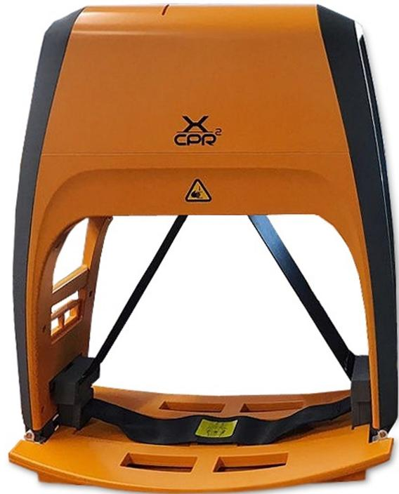
**FIGURE 1. Automatic SST-CPR device (X-CPR).** The main compression unit is positioned in the top of the device which is operated by a battery-powered motor. The strap is attached to both sides of the central piston.
