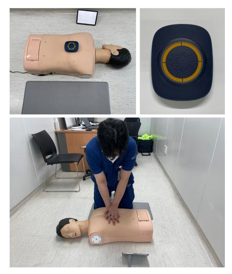
FIGURE 1. The cardiopulmonary resuscitation simulation manikin and the developed feedback device.
