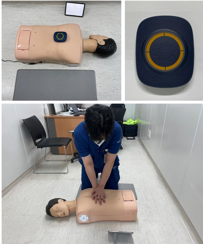
**FIGURE 1. The cardiopulmonary resuscitation simulation manikin and the developed feedback device.**
