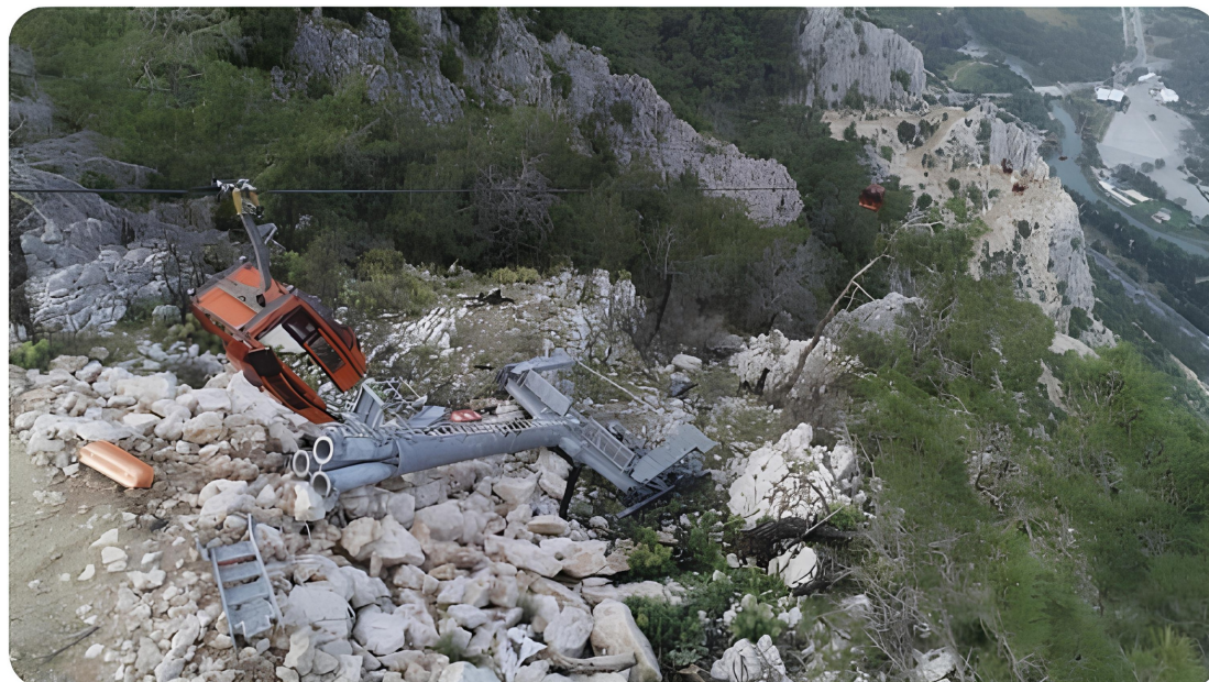
FIGURE 1. Image of broken cable car pole and falling wagon.
